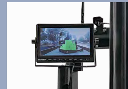
Camera systems for driving and pallet handling
