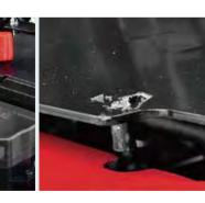
Integral locking pin structure on the baseboard can be opened without tool, which is convenient for daily repair and maintenance.
