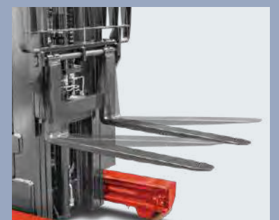
Forks can tilt forward/backward for easy loading
