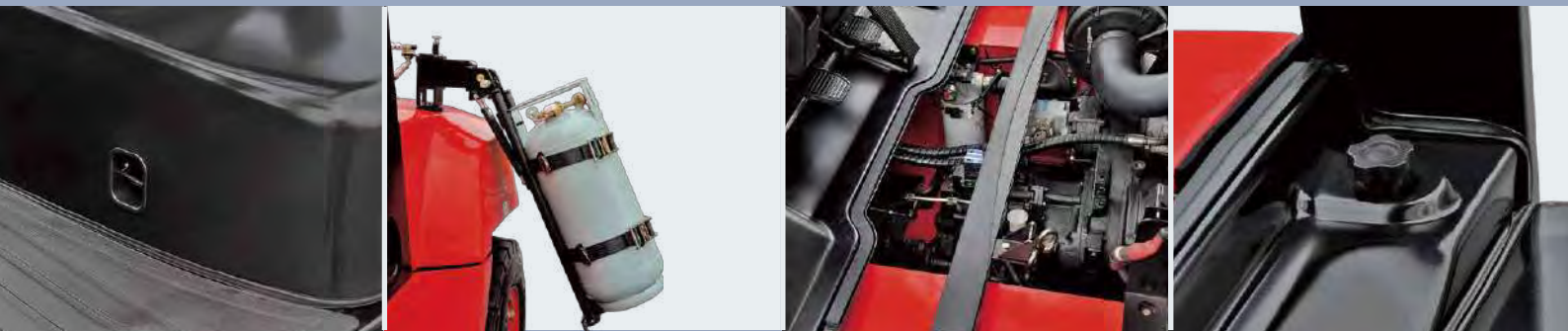
The location of the air-filter is easy to reach,and it's very easy to replace the filter.
