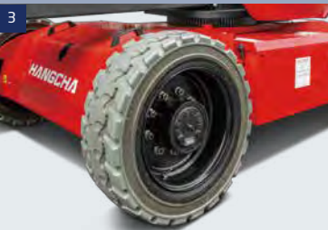
Tires: foam-filled tires with good off-road performance
