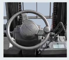
The design of steering wheel of small diameter and electro-hydraulic reversing as well as the car-type double-handle combination switch will greatly improve the driving comfort.
