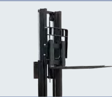
Mast tilting is the optional feature, offers proportional forward/backward speed
