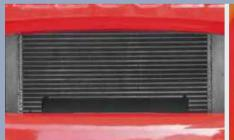
1. The radiator adopts aluminous plate-fin radiator with better performance and higher structural strength independent oil radiator, optimized oil and water heat dissipation channel and double ventilation holes on counterweight can greatly improve cooling efficiency and reliability of overloaded operation and ensure reliable operation of the engine.
