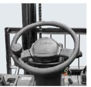
The design of steering wheel of small diameter and electro-hydraulic reversing as well as the car-type double-handle combination switch will greatly improve the driving comfort.
