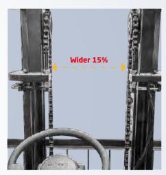
Adopt the new-type of box iron. Increase the inside width of inner mast and the spacing between lifting cylinders. The lowering of instruments in the driving cab will greatly increase the forward visibility; The rear visibility will also be greatly improved through the optimization design of counterweight.
