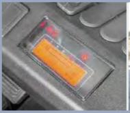
Newly-developed LCD instrumen has more comprehensive functions and more stable performance and entirely displays the full truck running state, trouble diagnosis and othe important information, which can make the operator more intuitively and conveniently have a better knowledge of truck state and make the maintenance conveniently.
