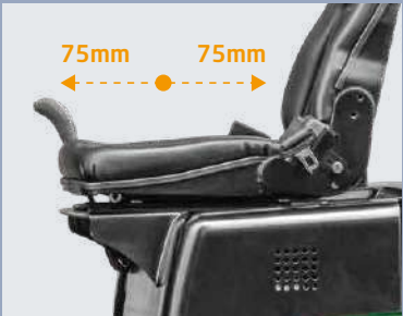
Seat can be adjusted backwards and forwards
