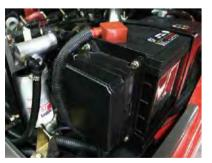
The new vehicle controller integrates all electrical components, features excellent durability for temperature, water and vibration for most demanding operation.
