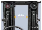
The developed front lifting cylinders with smaller outer diameter give the operator superior forward visibility.
