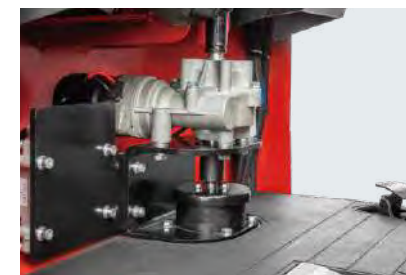
Electronic power steering system (for stand-up driving type tractor)
