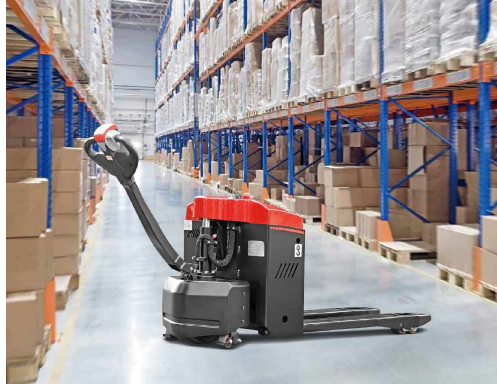
A Series Mini Pallet Truck with capacities of 2,000kg
